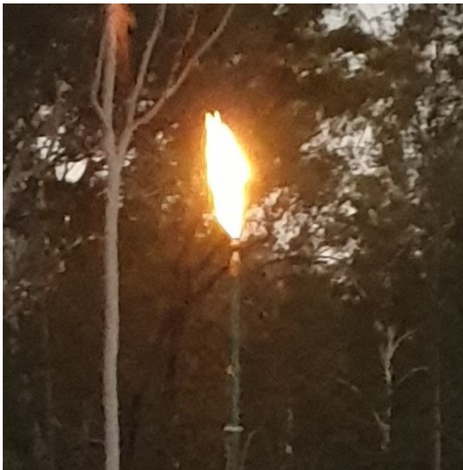
Gas flare at Serocold-1 on 27 July 2020 after de-watering for ten pumping days.
