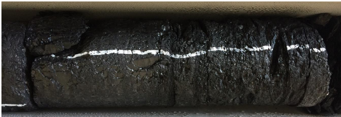
Reid's Dome Beds coal sample, Nyanda-4 showing fractures & cleating
