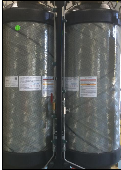
Above: Type 4 Carbon Fibre Cylinders similar to those being used in the State Gas Virtual Pipeline
